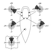
Be also aware that selftailing arm is positioned correctly. We recommend to have the selftailing arm positioned within the shaded area. On 12ST and 28ST the position of the selftailing arm is fixed, making it very important to establish the proper location of the holes prior to drilling these in the deck. On all other models, the selftailing arm can be placed in several different positions after having installed the winch.
