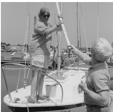
pushing extrusion up forestay
