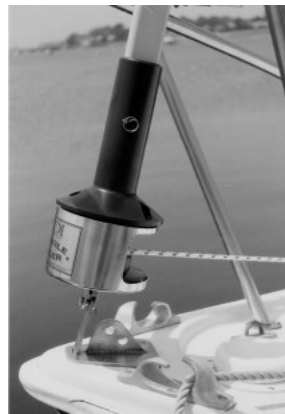
Furler w/ luff support pin installed
