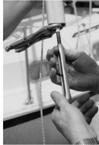
screwing TB on stud
