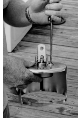
Assembling cup, bearing and antirotation strap
