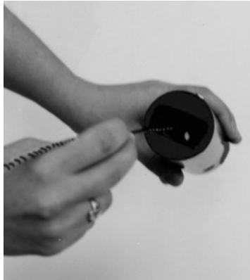
Inserting unfinished end of halyard into HTF (bottom view)
