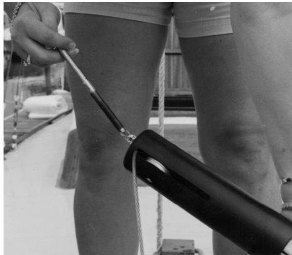
Connecting swage stud to messenger line
