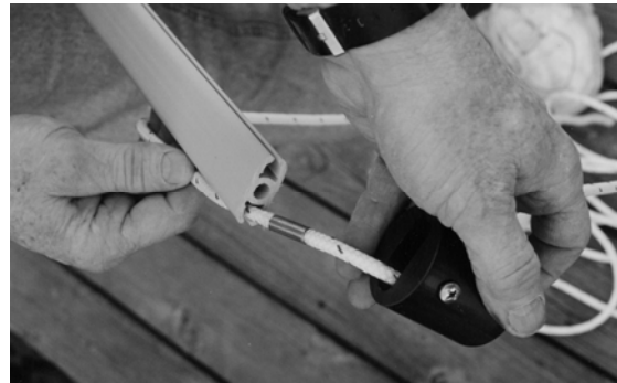
Pull halyard thru HTF. Ferrule gets inserted into the top of the luff extrusion.
