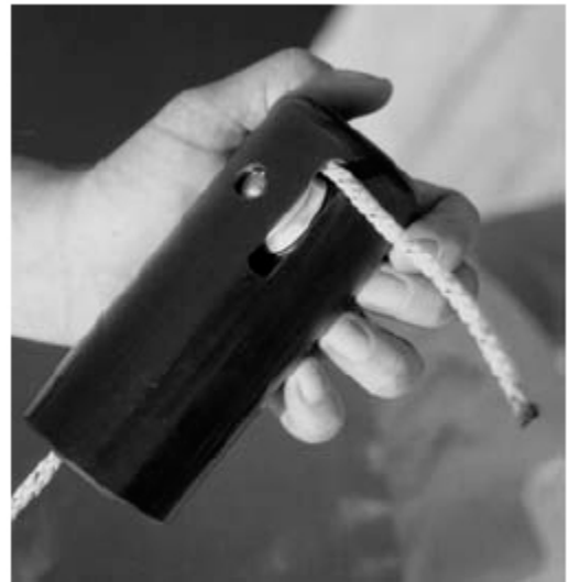
Rope halyard fed thru HTF & sheave (side view)
