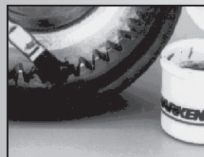
Use a brush to spread a light, even coat of grease.
