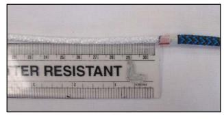
3. Remove 30cm of core from both ends (red and blue) of the rope.
