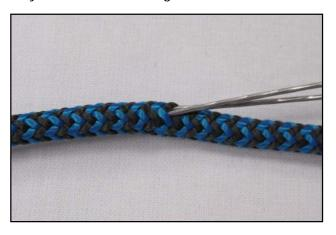
5. Insert the splicing needle at exact point that the core stops (mark B) and push down the inside of the cover and break out at mark A.
