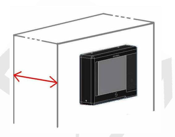
Wherever you mount the **NS-START POCKET** v², it shouldn't be flush to any thick surface such as the hull, so that the sensitivity of the embedded GPS receiver is not affected. Also a direct mount on a metal surface will reduce the receiver sensitivity.
