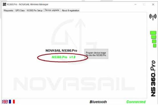
Once enabled in the setup parameters of the NOVASAIL Wireless Manager Windows or MAC software, the device will start transmitting the NMEA0183 data through Bluetooth.
