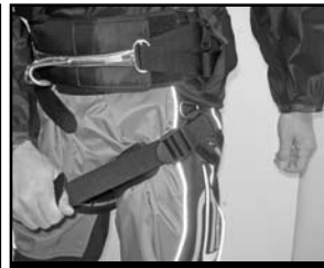
Tighten the leg straps to a snug fit.
