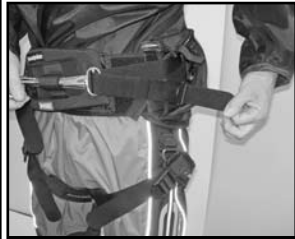
Bring spreader bar across and thread webbing through spreader bar end and back to buckle.
