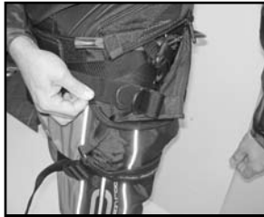
Double thread webbing in harness buckle. Lever buckle back and forth pulling the free end of the webbing to cinch harness tight.
